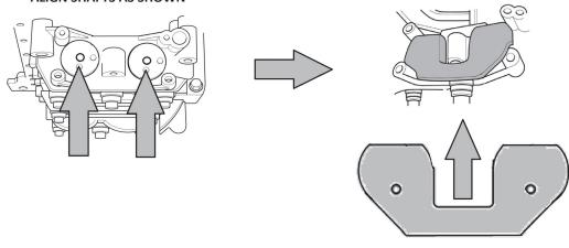
**Component B –** Balance Shaft Locking Tool Used to lock the balance shafts. Install as shown.
